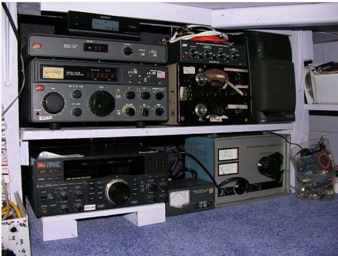
The Sony HD rx is on top of the classic NRD 515. The power unit bottom right is a variable supply useful for the required 110V
